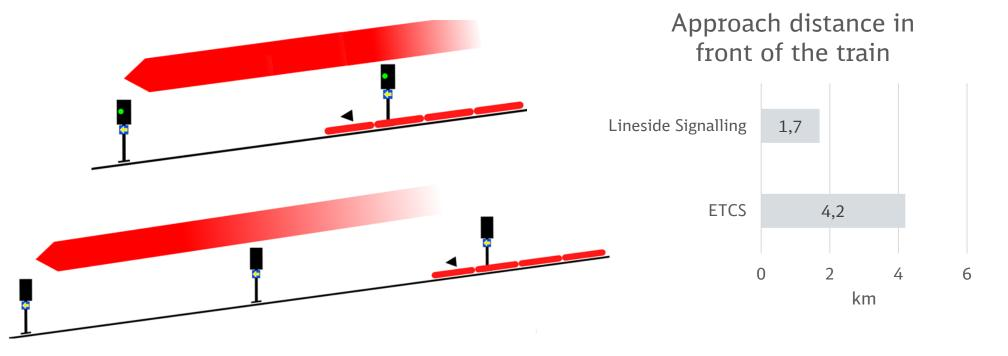
With ETCS, the train consumes significantly more capacity in the approach to Stuttgart central station than with lineside signaling.
