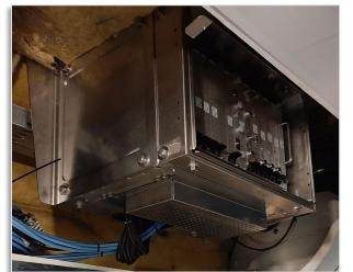
An ETCS/ATO computer (EVC) underneath the roof.
