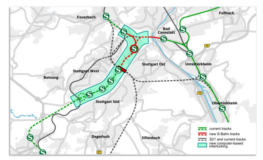
Figure: Core (*Stammstrecke*) of the Stuttgart S-Bahn system, including the control area of the new computer-based interlocking planed as of 2015. Further reading: *ETCS* as a carrier system for improved performance at S-Bahn Stuttgart. Signal+Draht 6/2019 (<u>https://bit.ly/2MJ4zAY</u>). Deutsche Bahn | Stuttgart | 2023-06-29
